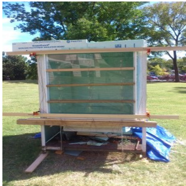
Figure 11. Picture of water-filled glazing unit with thermocouples attached.
