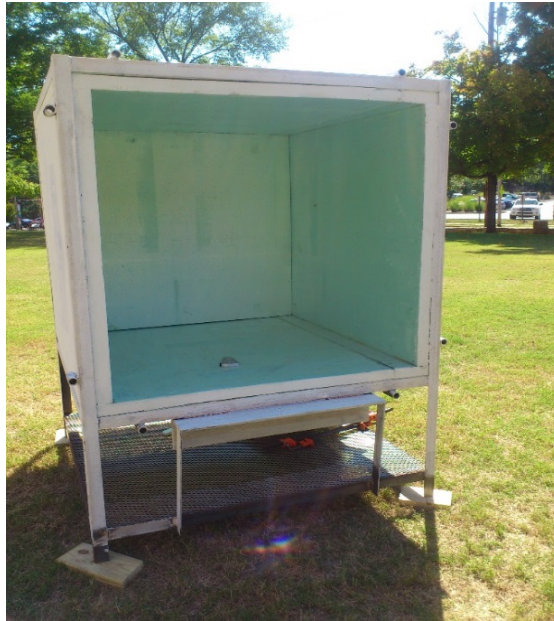
Figure 6. Fabricated test bench with an open aperture.
