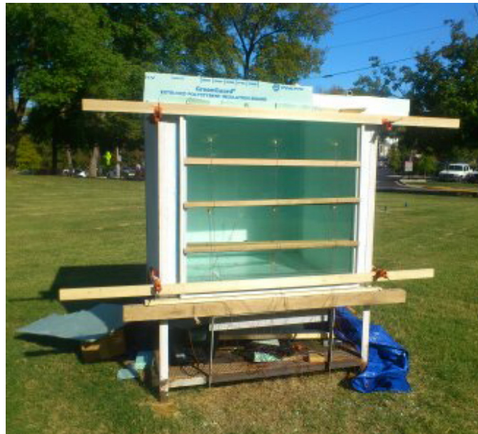
Figure 9. Picture of experimental setup 2 simulating air-filled glazing unit.
