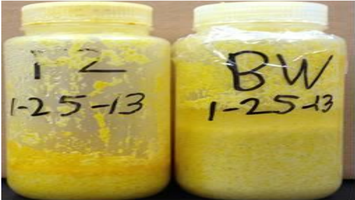
Figure 5.1 Raw fermenter and beerwell samples. These raw samples were collected from Commonwealth Agri-Energy, Located in Hopkinsville, Kentucky, Samples were immediately stored on ice upon retrieval, and were processed using the methods described in Section 4.1.
