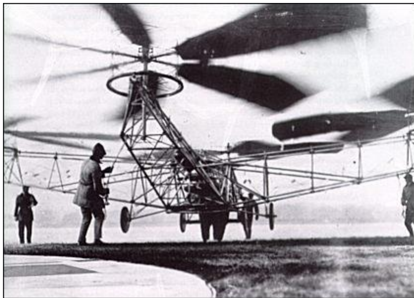
Figure 1: Dr. George de Bothezat and Ivan Jerome developed the manned quadrotor shown above in 1922 [1]
