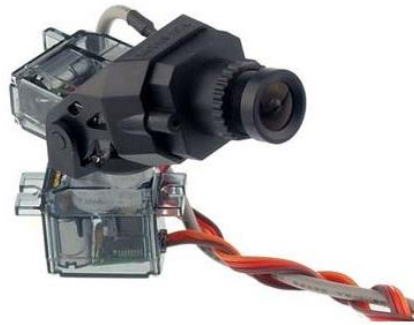
Figure 10: A premade pan/tilt camera used for FPV and co-axial camera views. The official title for the camera system is “600TVL FPV Tuned CMOS” (TVL: Television Line, FPV: First Person View, CMOS: Complementary metal–oxide–semiconductor [8])
