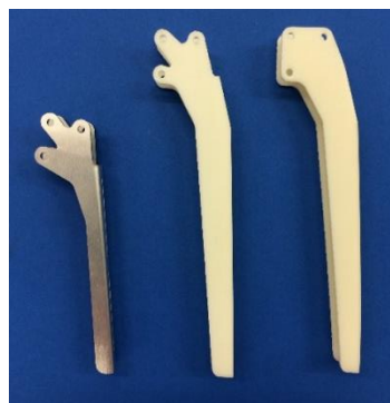
Figure 9: Landing gear design iterations from left to right: Aeroquad stock gear, first design iteration, second and current design iteration
