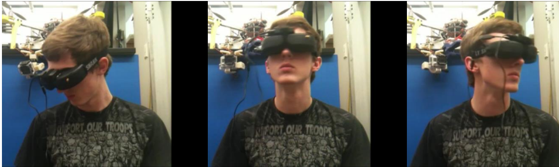
Figure 16: Demonstration of camera orientation control using a head tracker sensing user movement
