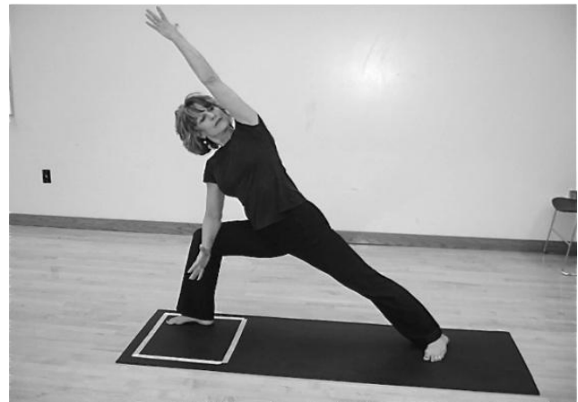
Figure 1. Condition 1. Force plate perimeter is outlined on yoga mat and subject begins sequence by standing over the force platform. Forces are measured in either one or both lower and upper extremities.
