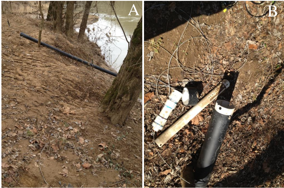
Figure 7- (A) Munfordville data logger site, (B) PVC encasements for data loggers. Source: Photo by the author.
