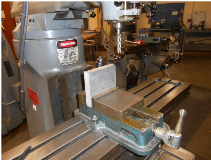
Figure 2. Aluminum block with factory edge against base of vice.
