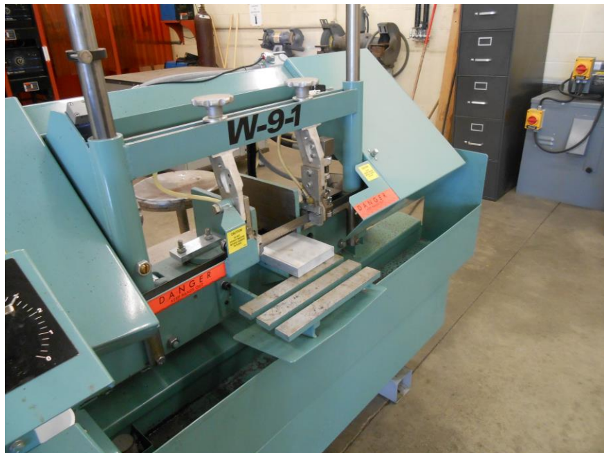
Figure 1. Horizontal bandsaw used to cut aluminum flat stock.
