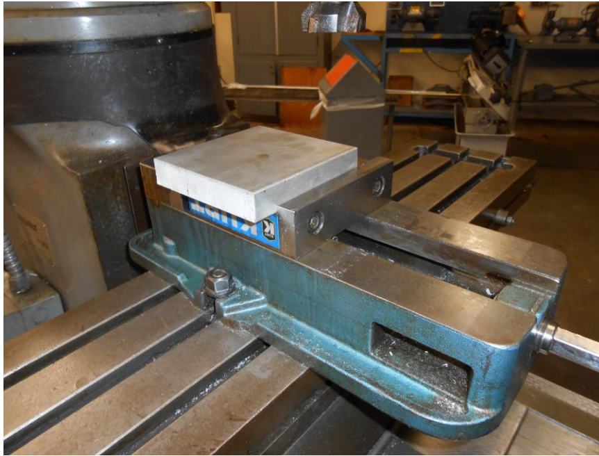
Figure 3. Clamping position to machine first Y axis.
