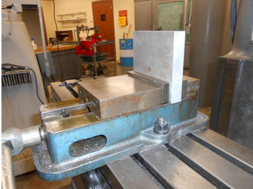
Figure 4. Processing final Y axis with aluminum block placed vertically in vice.
