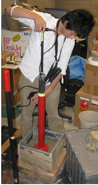
Figure 2: Picture just prior to impacting surface with Clegg Hammer.
