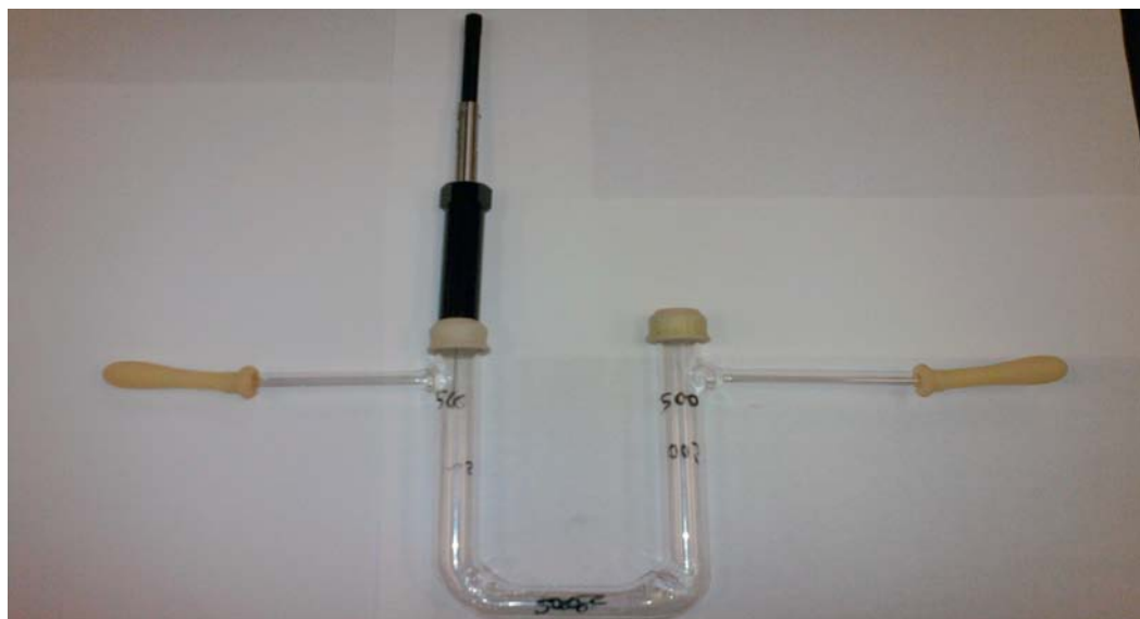
Figure 2.5. Adsorption of the volatile substances by SPME fiber
