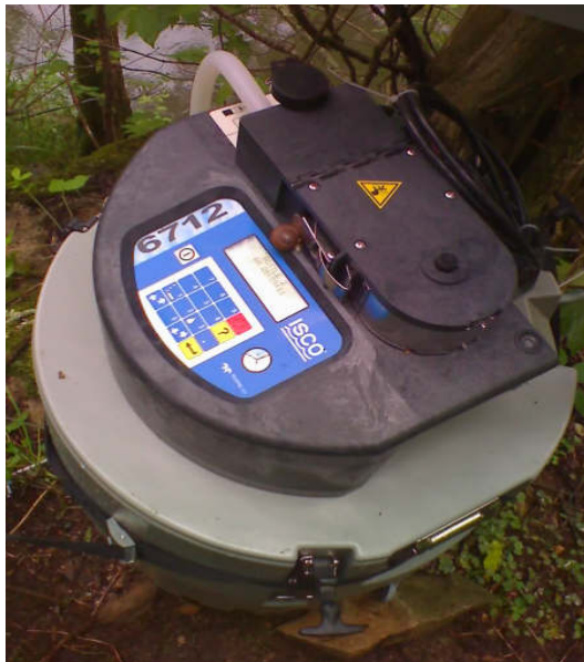
Figure 4.6: 6712 ISCO portable water sampler used in the research
