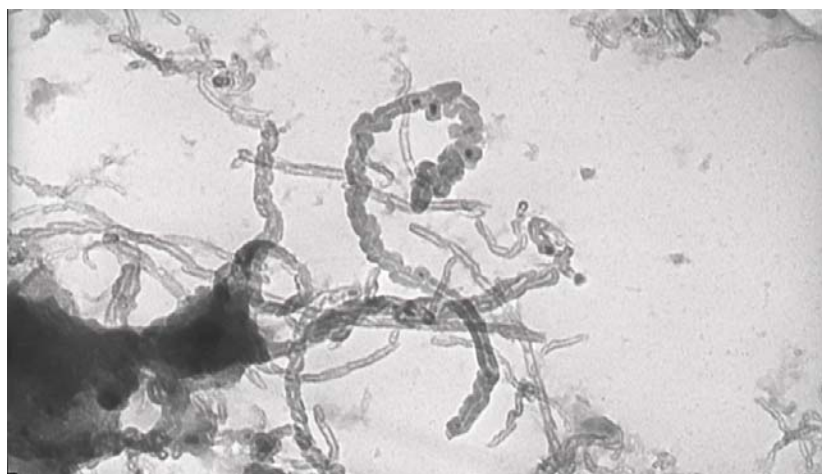
Figure 4.1a: Raw Commercial MWNTs
