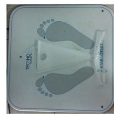
Figure 2: COG sensor used during the experiments.
