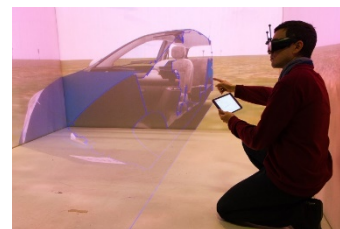
Figure 3: VARI3 allows a user to manipulate a virtual model using a tracked handheld tablet.
