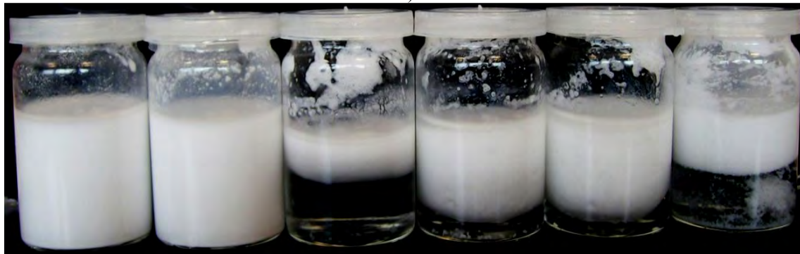
Figure 5: Oil water emulsions obtained for different values of ionic strength. a) initial emulsion; b) emulsion after 10 days rest.
