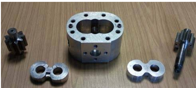
Figure 7 Real gear oil pump components
