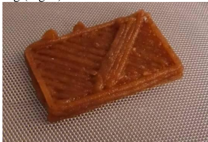
Fig 3. First reconstituted wood model by additive manufacturing
