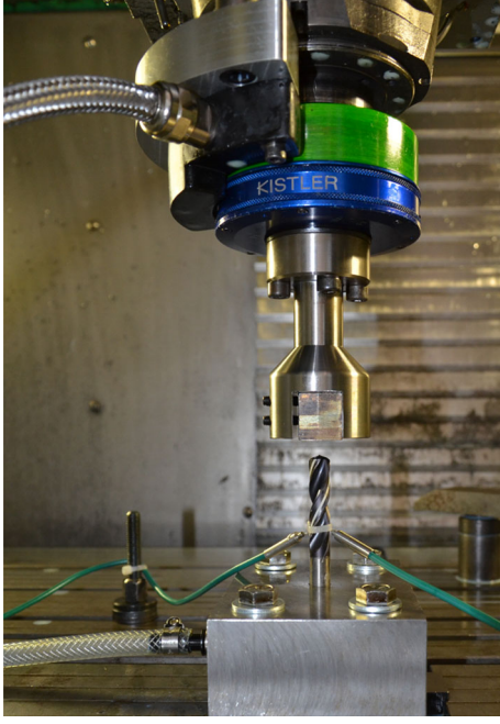
Fig. 4 Experimental set-up for temperature measurement
