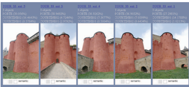
Figure 9. Entity-based images searching in the 3D scene. When one or more 3D entities are selected in the 3D scene, all photographs in which these elements are present are listed. The semantic layer related to the selected elements (mapped on photos as a SVG mask) is highlighted.
