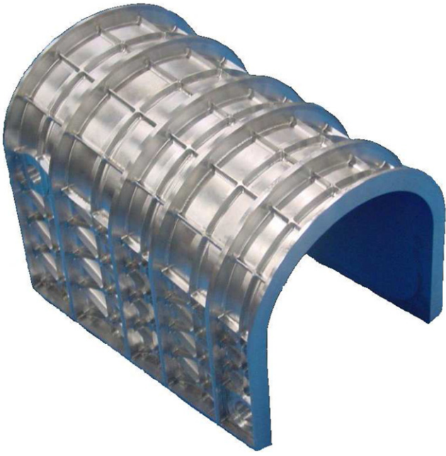
Fig. 10. Manufactured prototype of the landing gear compartment. The studied parts are the inner surfaces of the structure.
