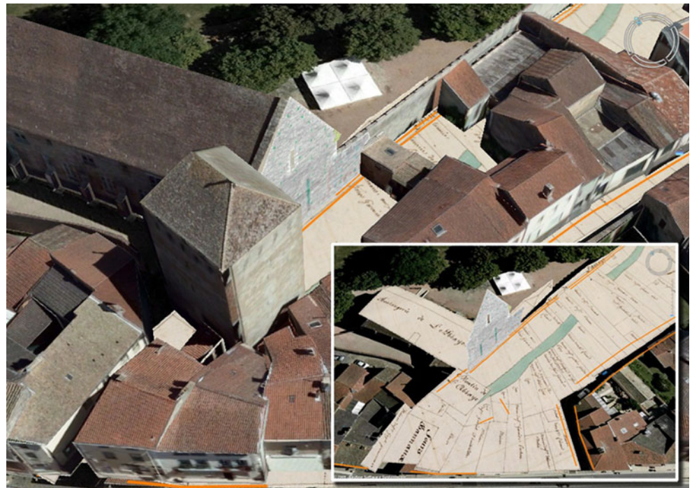
Fig. 7 Mill Tower: today's city (3D CAD model) and the eighteenth century plan as under layer to understand the evolution of the city
