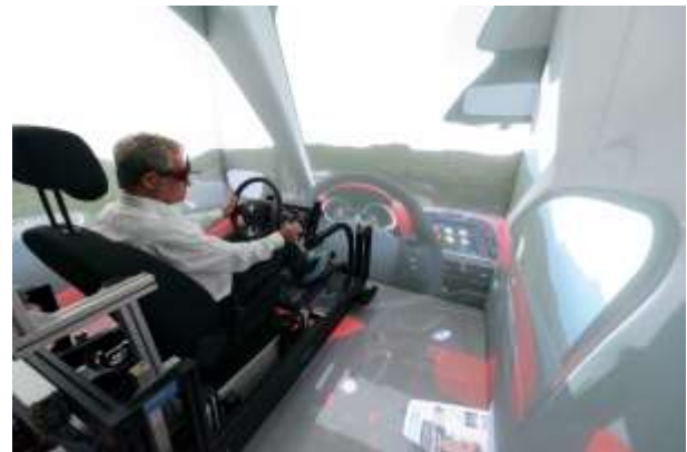
Figure 5. Renault's high performance CAVE™ with driver station
