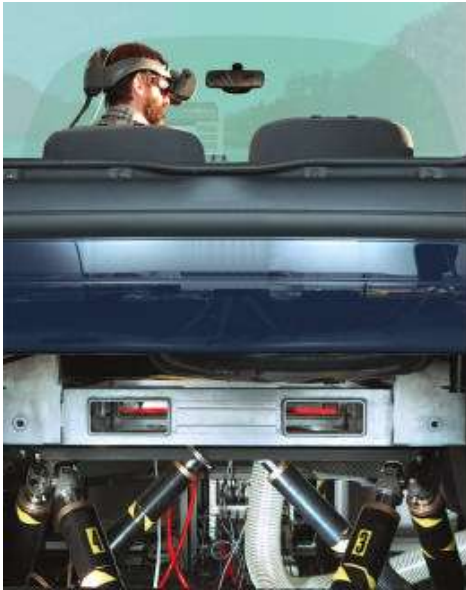
Figure 1. HMD equipped motion based simulator prototyping, CARDS © Renault
