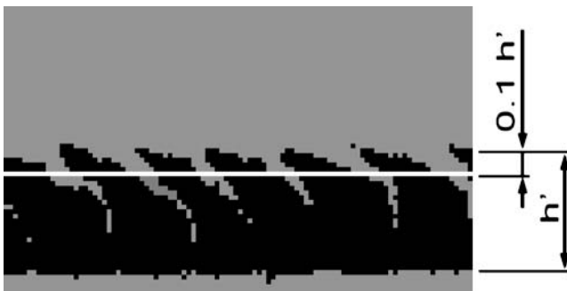
Fig. 6 Rescaled image of veneer used for Region Of Interest (ROI) extraction and coarse positions of checks determination at the specified depth of veneer – 10% of its thickness ( h' )
