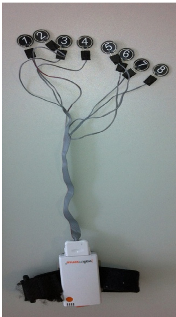
Figure 2 Walkinsense equipment. Sensors are 1 cm 2 and <1 mm thick.
