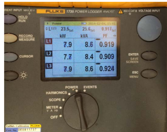
Fig 4. IE 3 Motor Power measurement at 50 Hz
