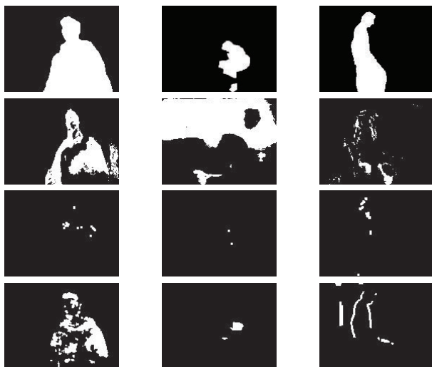
Fig. 4: Foreground segmentation masks of proposed solutions. The columns correspond to the "Waving Trees", "Time of Day" and "Light Switch" sequences respectively. The first row represents the ground truths while the remaining rows correspond to the outputs of the solutions proposed by Zhou et al. , Ng et al. and Vemulapalli respectively.
