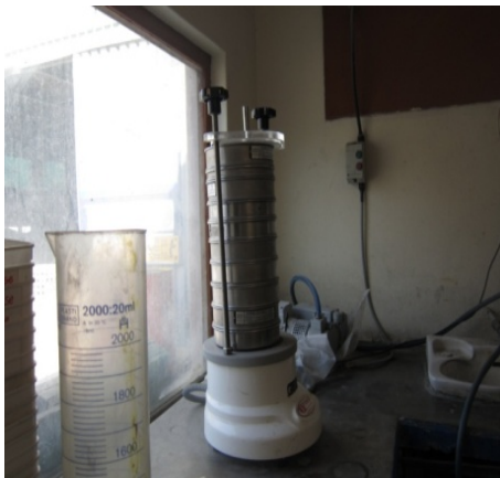
Fig. 6: Vibrating shaker used for particle size analysis
