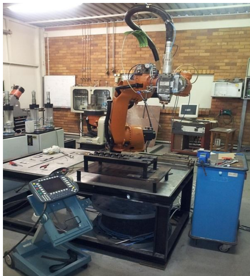
Figure 2: Experimental setup for LBF of Ti6Al4V
