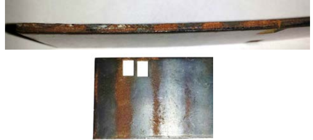
Fig 4. Rusted non-laser contacted regions
