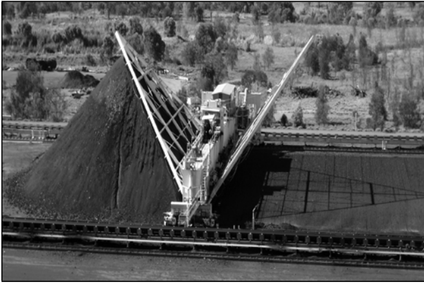
Figure 2. Stockpile discharged by using a Krupp bridge reclaimer at RTCA Kestrel Mine
