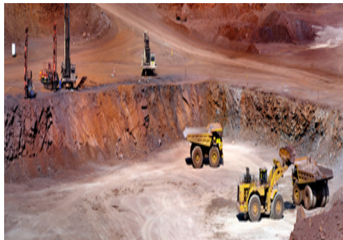
Figure 1. A mining operation of an iron ore mine, including drilling; explosion; loading; and hauling
