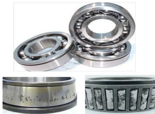
Fig. 1 Illustration of new and failed steel bearings, due to the damaged on the surface
