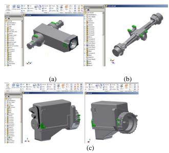
Fig. 2 3D Models of: (a) Transaxle, (b) Steering Axle, (c) Engine
