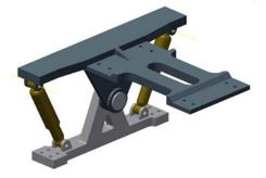
Fig. 3 3D Models of the front suspension assembly
