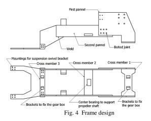
The second panel is bolted into the first one and has welded brackets on the inside for the front side of the engine mounting. The proposed design of the frame is shown in Fig. 4. The center bearing on Cross member 2 does not form part of the frame. It is inserted in the drawing to show the location of it and that it is going to be fixed on that particular cross member. The material for the frame is Weldox 700 that is a general structural steel with 700 MPa yield strength
