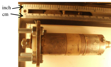
Figure 3: T&M Research Products co-axial current shunt resistor
