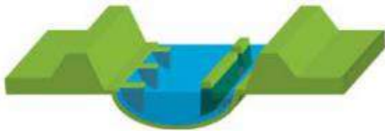
Figure 1: Cross section of a river with on the left bank traditional groynes and on the right bank a longitudinal training dam.
