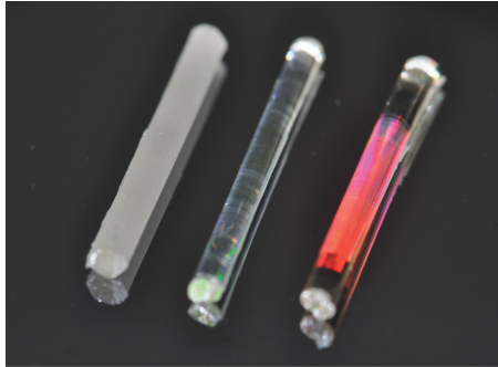
Figure 2: The produced curved rods with topographies (from left to right: Rough, 150 nm grooves, 200 nm grooves). The light breaking effect of the patterns allowed a fast elimination of implants having not properly replicated topographies. In the next step the implants were shortened to the necessary dimensions.
