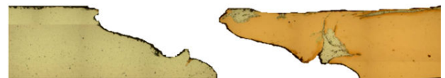
Fig. 3 (a) Fractured surface of weld produced at 950 rpm and 300 mm/min with the 25 mm shoulder diameter tool
