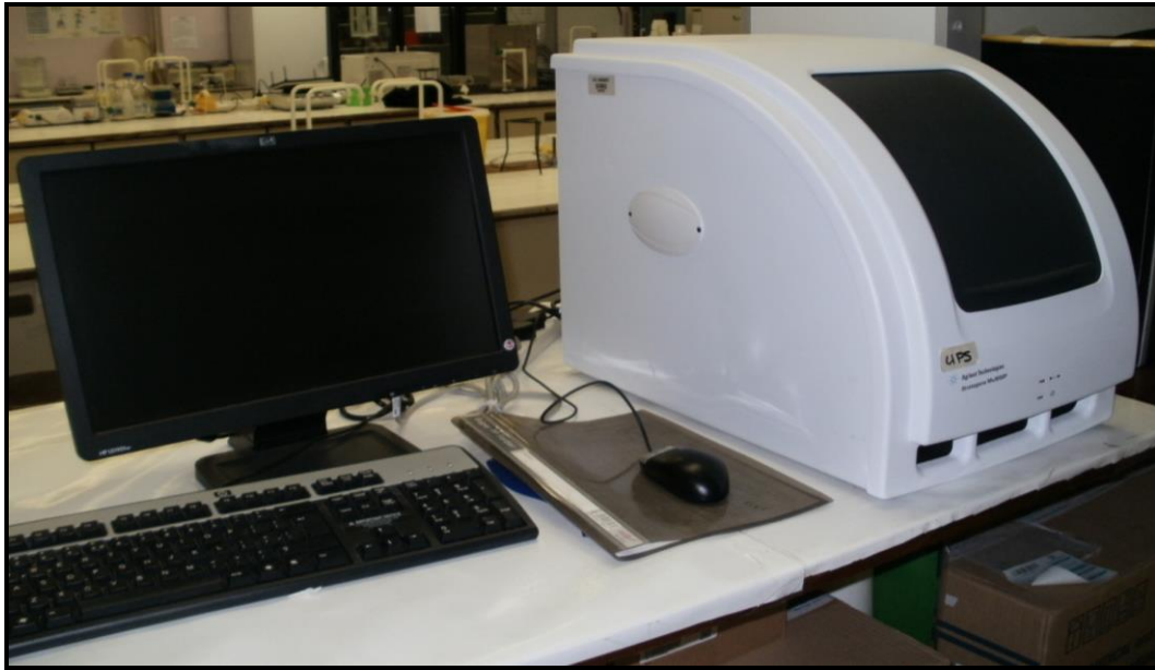
Figure 16. Stratagene Mx3000p ® used to analyse the expression of the genes from the cDNA of the co-cultures.
