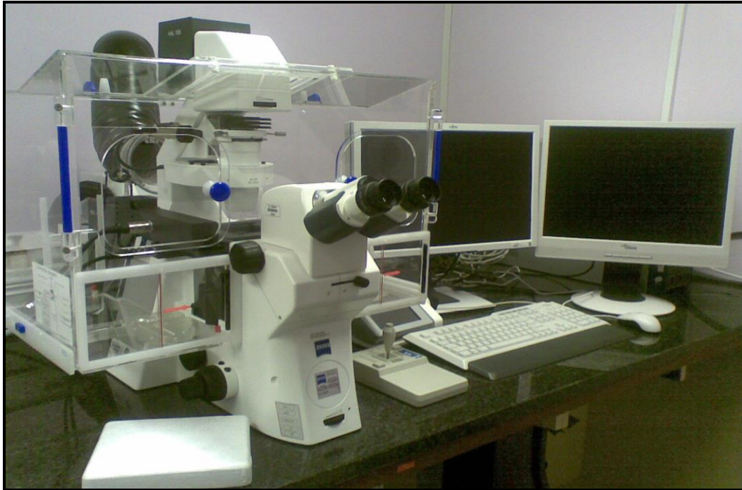
Figure 11. Expression of the markers through immunofluorescence was observed by the Carl Zeiss, Axio Observer Z1. The microscope was also used to get direct interference contrast images of the co-cultures.
