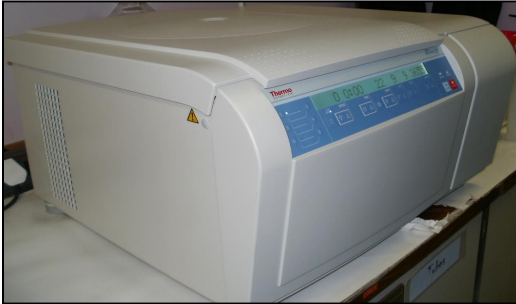
Figure 6. Heraeus megafuge 16R centrifuge used to spin cell suspensions.
