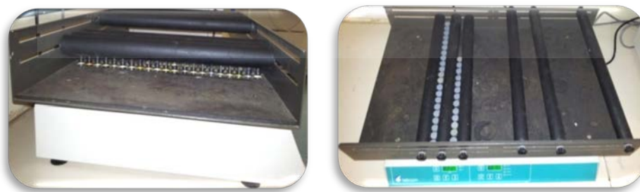
Figure 6.2 Side view ( left ) and front view ( right ) illustration of extraction of bio-wipes on a bench shaker.
