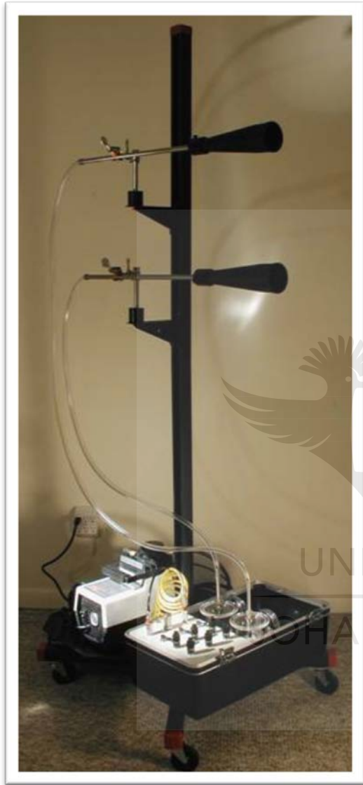
Figure 7.6: Helium Bubble Generator System
