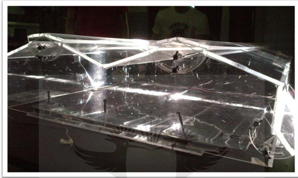
Figure 7.9: Helium Bubble Flow Visualization
