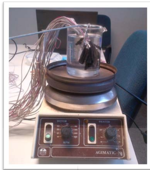
Figure 7.4: Calibration of Temperature Transducers
