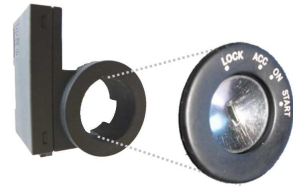
Figure 7.2: Immobilizer unit around the ignition barrel
