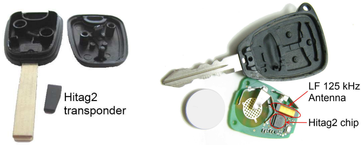
Figure 7.1: Car keys with a Hitag2 transponder/chip
