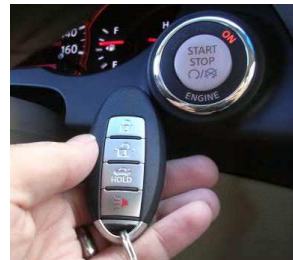
Figure 7.3: Keyless hybrid transponder and engine start/stop button
