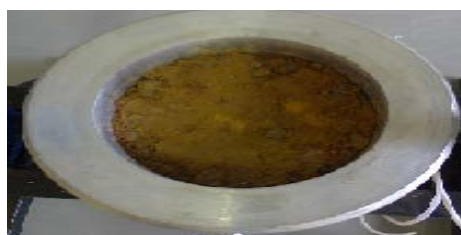
Figure 3 Thin soil layer overlying the CDW fitted in the bucket section as used in the study
