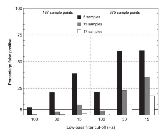
Results of the simulations for signal's length of 187 (left) and 375 (right) sample points with critical-run values of 5, 11, and 17 samples. Horizontal solid lines indicate the 5% critical alphalevel. 100 Hz = data filtered only during recording (0.016–100 Hz band-pass) with no additional low-pass filtering.
