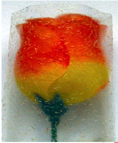
Figure 1. Photograph of flower wrapped with Cellulose/Thespesia composite film loaded with 5wt.% fibers
