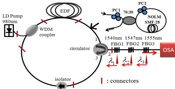
Figure 1: Schematic diagram of the experimental setup of the proposed three wavelength laser and the NOLM; PC: Polarization controller.
