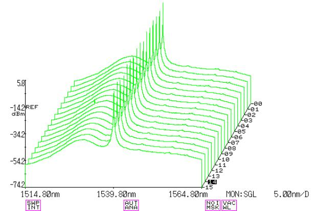
Figure 2: Spectrum of the laser without NOLM
