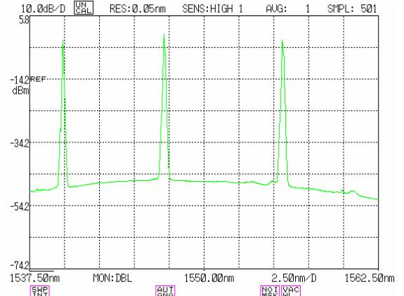
Figure 5: Spectrum of the laser with 2.5km of NOLM length in the laser cavity
