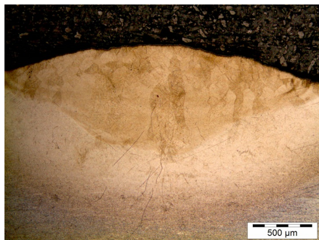
Figure 7 Micrograph of LMD sample at laser power of 800 W and scanning speed of 0.005 m/s showing no porosity
