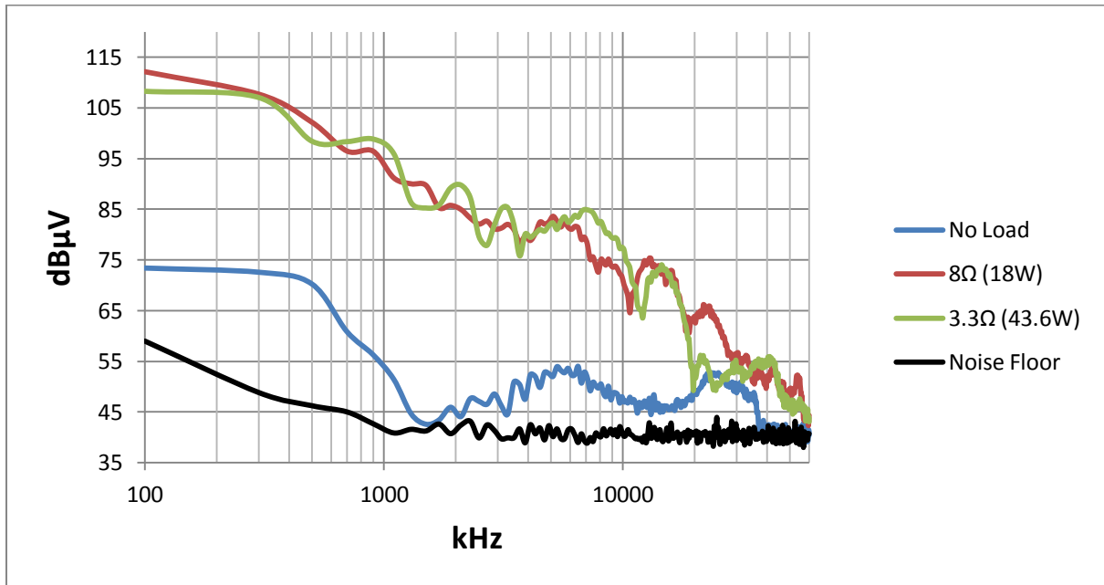
Figure 6-11 PCB3 Zero Elevation CM Results
