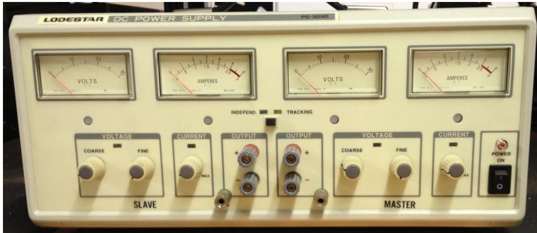
Figure 5-1 Linear DC Power Supply
