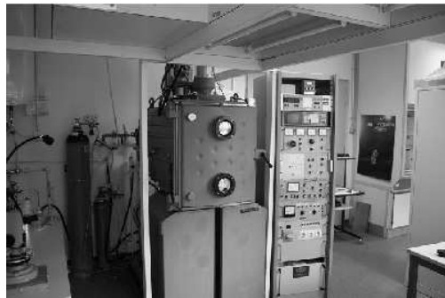
Figure 2: The Balzers BA k 550 vacuum chamber at the IAAT.
