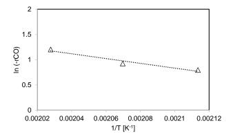
Fig. 4 Arrhenius plot for CO conversion
