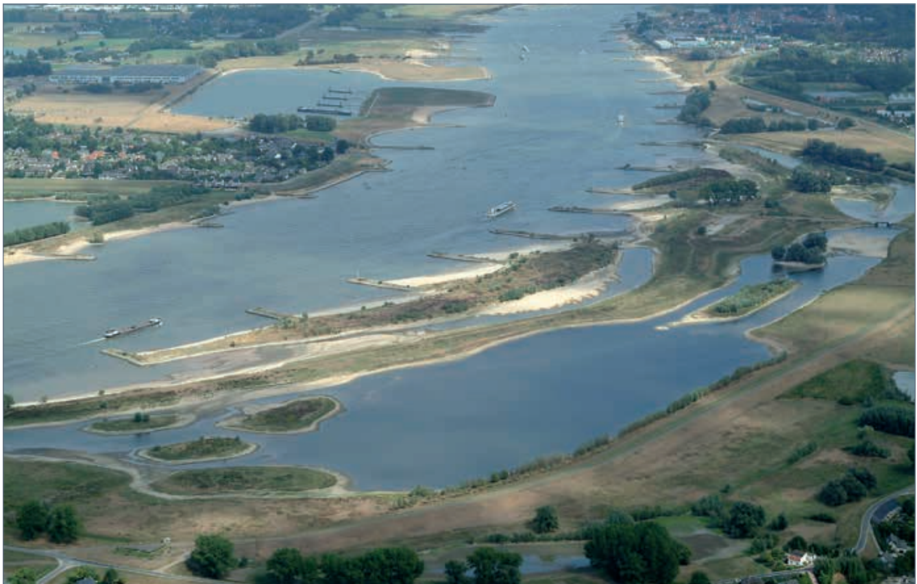
A secondary channel, parallel to the main channel in the Waal River, intended to spur nature development and reduce peak water levels
