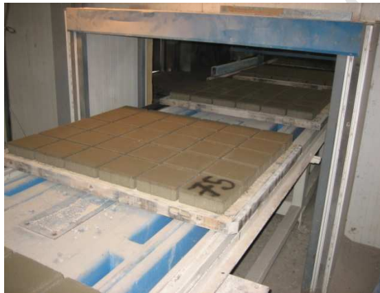
Fig. 4. Manufacture of pavement blocks.
