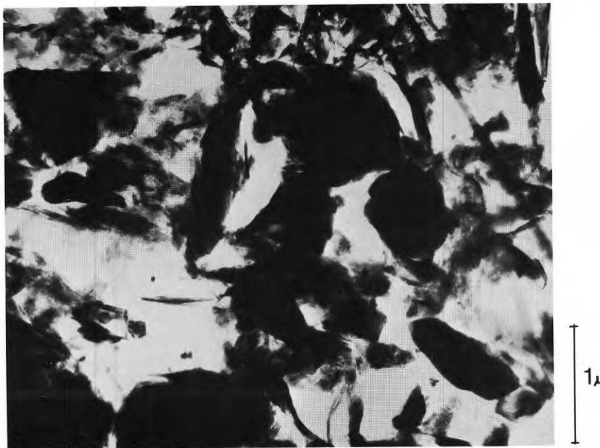
FIG. 1. Electron micrographs of ultra-thin sections of soft, illitic marine Lilla Edet clay.
